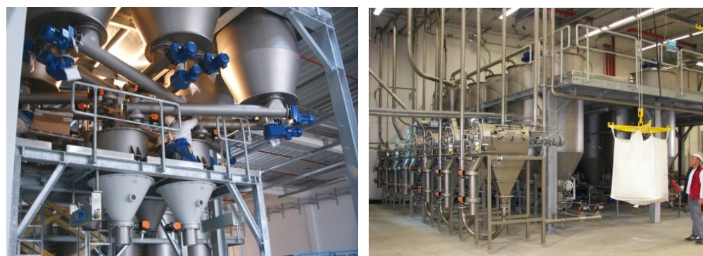
Reimelt weighing station and rotary sifters
